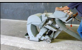
Before and after shot blasting...the profile after should be a little rough. We should discuss with the contractor and make sure that we get the largest machine possible for the project...ask the question as this will impact your schedule if you allow a small machine on site...a small machine is 9"...a good size should just be able to fit through the door.
